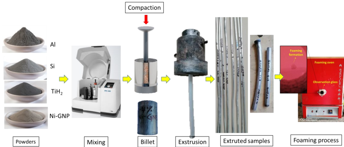
Figure 2. Schematic representation of the fabrication process of Ni-GNP/AlSi12 composite foam
