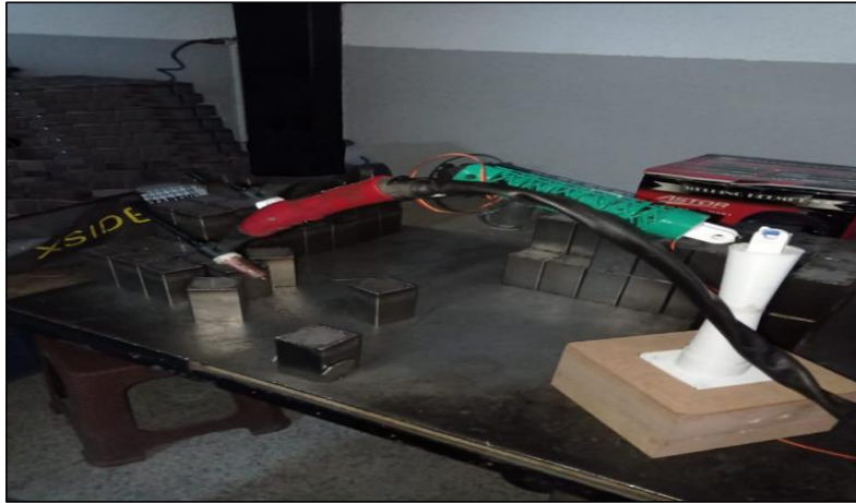
Figure 17. Starting position of welding torch
