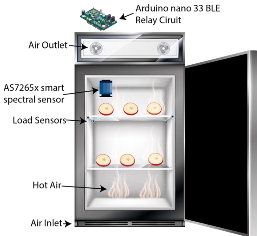
Figure 3. Edge Computing Supported Drying Cabinet and Components
