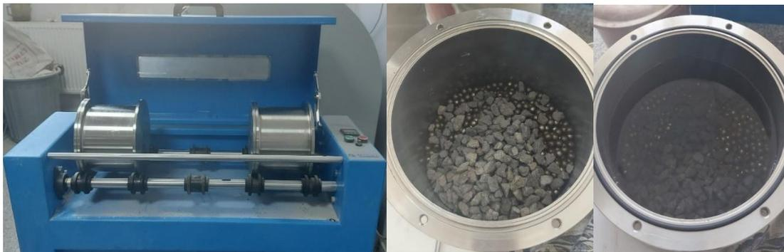
**Figure 5.** Micro-Deval Device, Micro-Deval drum, aggregate, steel shot and water mixture
