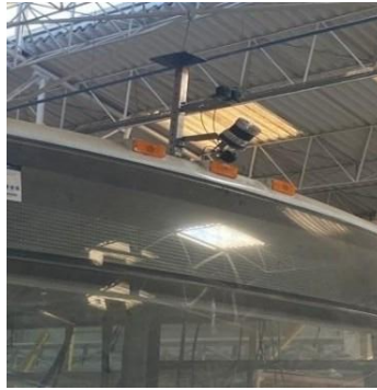
Figure 10. Integration of Lidar and Camera verse into vehicle superstructure (Camera at the top, Lidar at the bottom)
