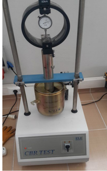
Figure 3. California bearing ratio test device
