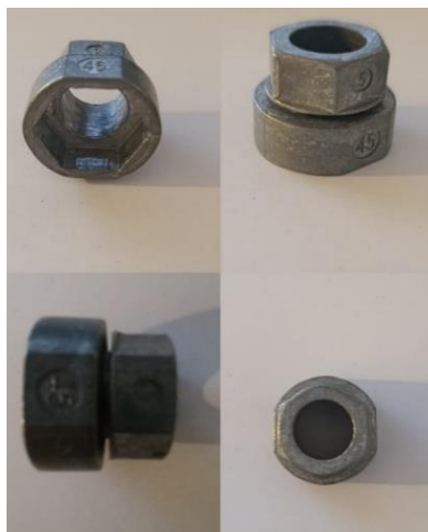
Figure 12. Adjustable bolt head samples post-die casting
