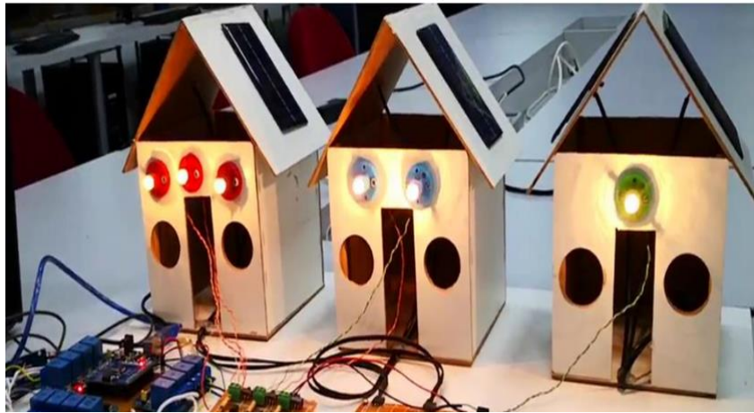
Figure 2. Three-unit physical prototype. The house models make renewable generation, storage, and load use visible.
