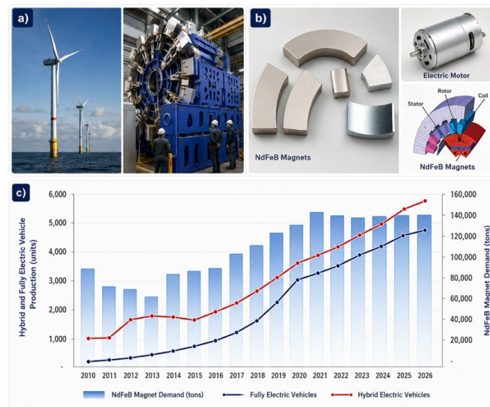
Figure 3.8. a) Application of NdFeB permanent magnet generators in wind turbines; b) Various application areas of NdFeB magnets; c) NdFeB magnet demand in hybrid and fully electric vehicles (2010–2026) [2]
