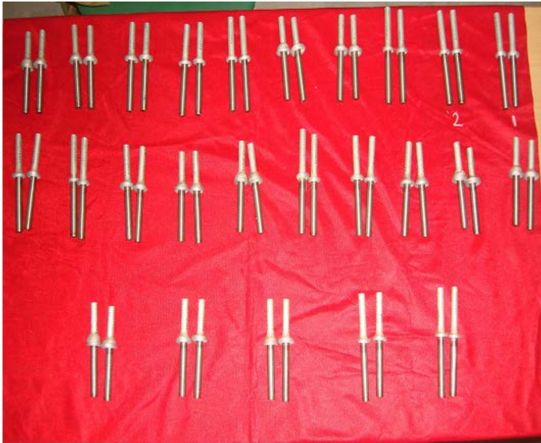
Fig. 3 Photograph of Friction welded ASS-Al Joints
