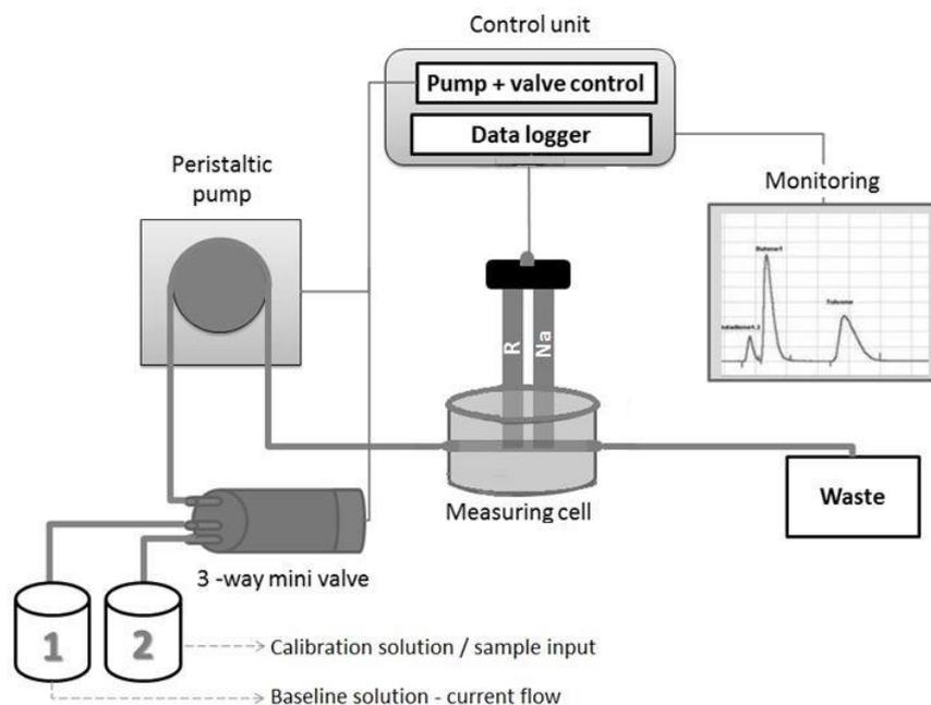
Figure 1. The scheme of the flow system that uses Na ion selective electrode as detector.
