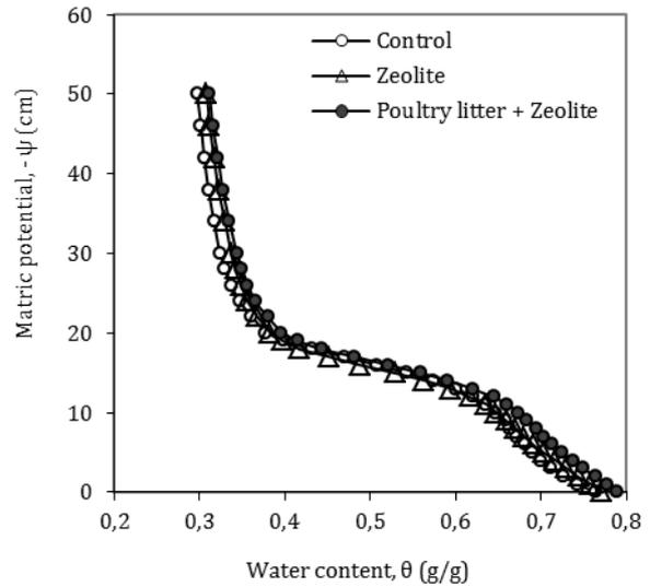
Figure 4. Clay soil water retention as affected by poultry litter and zeolite application under wheat
