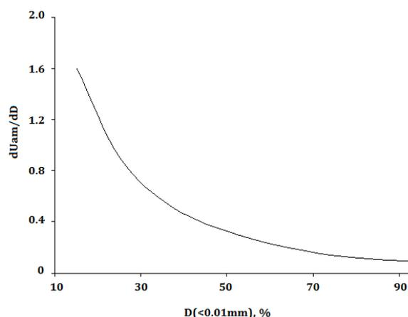
Figure 3. The change rate of moisture content ( $dU_{am}/dD$ ) depending on clay particle content in the soil.
