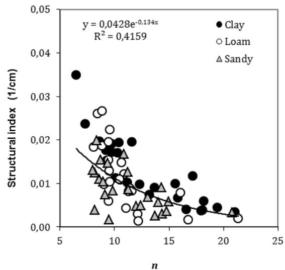
Figure 8. Soil structural index (SI) as a function of  $n$  for soils (clay, loam and loamy sand) treated with composted manure and sewage sludge and their components (orthophosphate, phytic acid and humic acid)
