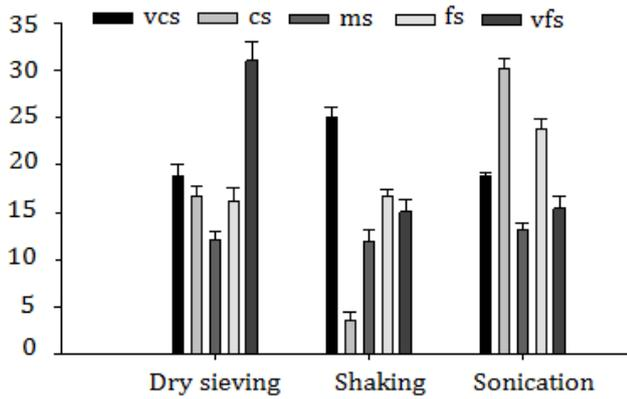
Figure 6. Sand fraction distribution after applying disaggregation methods in horizon Cky (5-35 cm) from profile 5. Shaking -15 hr shaking in 7:3 ethanol: water solution; sonication- sonication for 3 min. in 7:3 ethanol: water solution.
