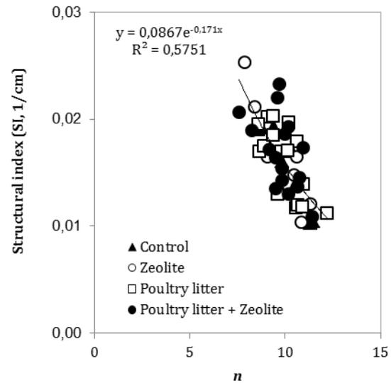
Figure 12. Soil SI as a function of  $n$  for clay soil treated with poultry litter and zeolite, and their combination
