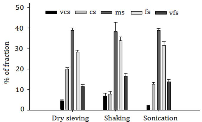
Figure 4. Sand fraction distribution after applying disaggregation methods in horizon Czy (5-25 cm) from profile 3. Shaking -15 hr shaking in 7:3 ethanol: water solution; sonication- sonication for 3 min. in 7:3 ethanol: water solution.
