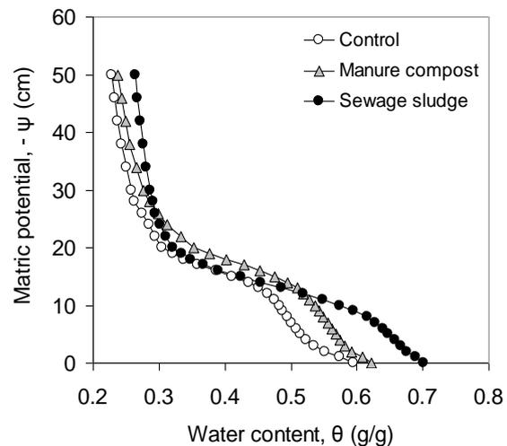
Figure 2. Loam soil water retention as affected by composted manure and sewage sludge application
