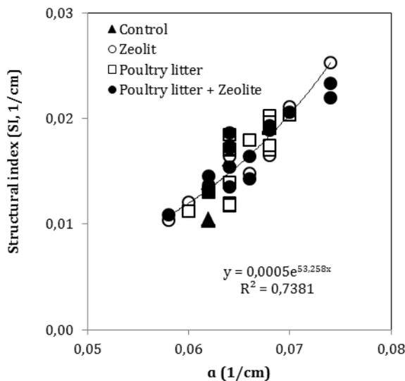
Figure 11. Soil SI as a function of  $\alpha$  for clay soil treated with poultry litter and zeolite, and their combination.
