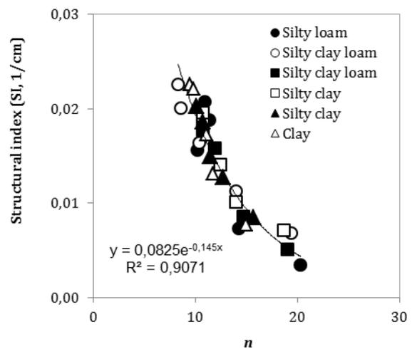
Figure 6. Soil structural index (SI) as a function of *n* for six soils (ranging from loamy sand to clay) saturated with five wetting rate (2, 8, 32, 100 and 200 mm h<sup>-1</sup>)
