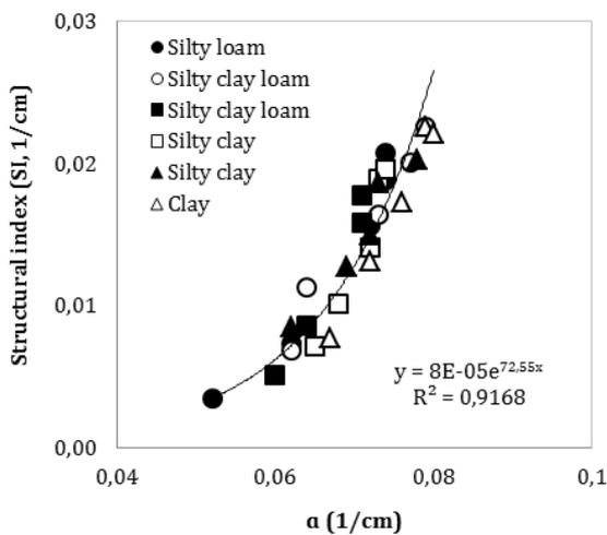
Figure 5. Soil structural index (SI) as a function of  $\alpha$  for six soils (ranging from loamy sand to clay) saturated with five wetting rate (2, 8, 32, 100 and 200 mm h<sup>-1</sup>)
