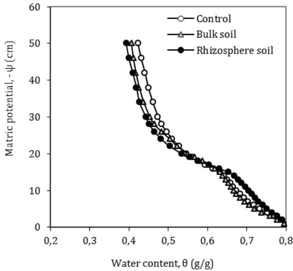
Figure 3. Clay loam soil water retention (control, bulk and rhizosphere) as affected by cropping under wheat
