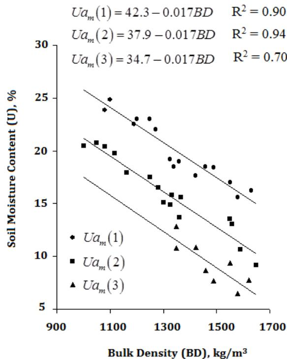
Figure 2. The moisture content corresponding to the maximum thermal diffusivity values of the soils of clayey (I), loamy (II) and sandy loam (III) particle size distribution depending on the bulk density.
