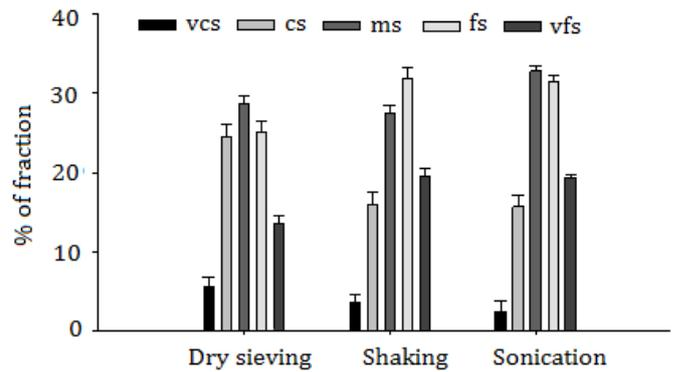
Figure 2. Sand fraction distribution after applying disaggregation methods in horizon Czy (5-25 cm) from profile 1. Shaking -15 hr shaking in 7:3 ethanol: water solution; sonication- sonication for 3 min. in 7:3 ethanol: water solution.
