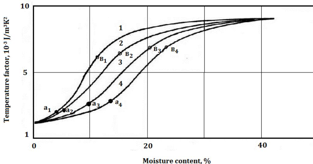
Figure 1. Temperature factor dependence of the volumetric thermal capacity of silica sand (1), sandy loam (2), loam (3) and clay (4) depending on moisture content
