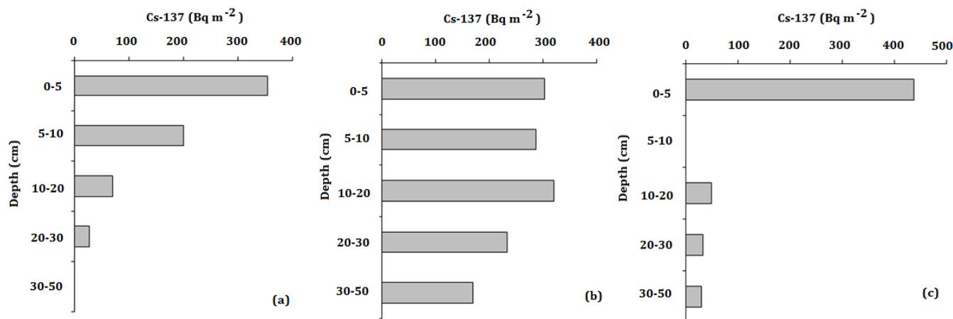
Figure 3. Vertical distribution of <sup>137</sup>Cs (Bq m<sup>-2</sup>) at site X<sub>3</sub> (a), site X<sub>11</sub>(b) and site X<sub>14</sub>
