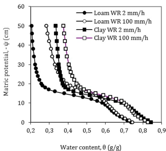
Figure 1. Soil water retention as affected by wetting rate (WR)
