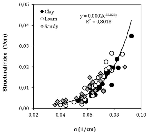
Figure 7. Soil structural index (SI) as a function of  $\alpha$  for soils (clay, loam and loamy sand) treated with composted manure and sewage sludge and their components (orthophosphate, phytic acid and humic acid)
