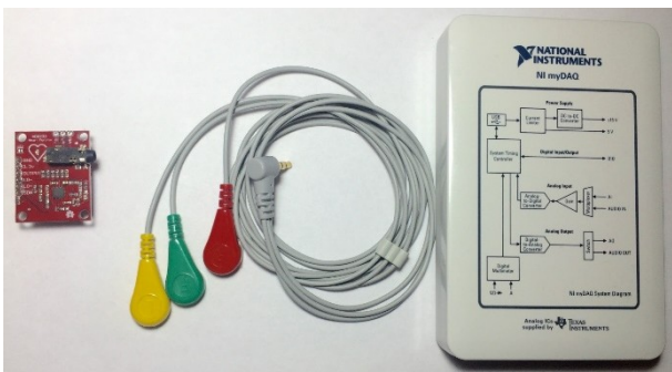
Figure 3. AD8232 ECG module and NI myDAQ card
