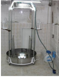
Figure 1. General view of rainfall simulator
