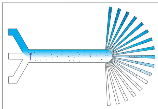
**Figure 5:** Microfluidic device to increase the concentration of bacteria by chemotaxis in different channels. Figure adapted from (27).
