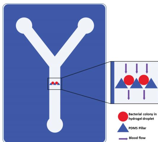
**Figure 3:** Microfluidic device for objective 1
