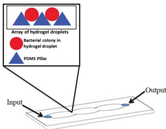
**Figure 8:** Design in the microfluidic device mimicking the *tortuous* flow of blood as in venous stasis cases
