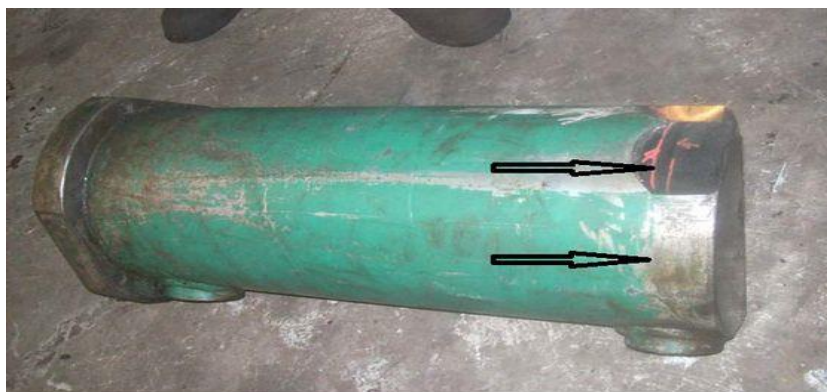
Figure 1. General view of the broken cylinder bushing
