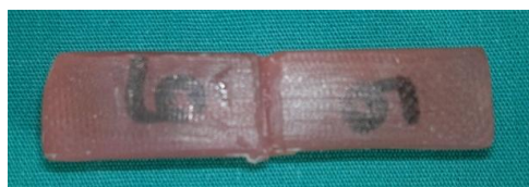
Figure 3. The soft lining materials between the specimens
