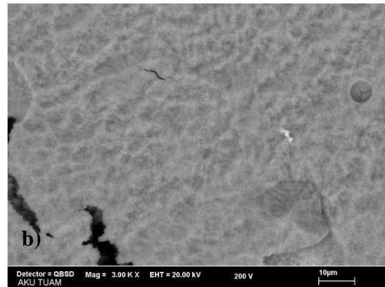
Figure 7. Supply voltage of 160 volts) optical microstructure b) SEM image of avulsion fracture surface
