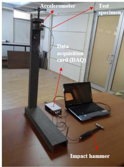
Figure 2. Vibration test set-up. (a) Sketch of vibration test mechanism and unbonded-one piece specimen, (b) Overall view of vibration set-up
