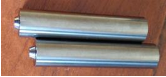
Figure 2. Tapered pin having 3.2 mm and 3.5 mm length of friction stir spot welding tool
