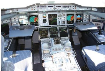
Figure 21. The Airbus A380 glass cockpit featuring "pull out keyboards and 2 wide computer screens on the sides for pilots" [85].
