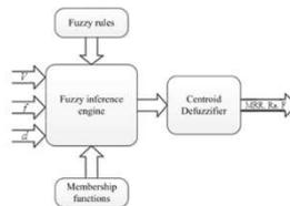
Figure 2: 3-inputs and 3-outputs fuzzy logic system
