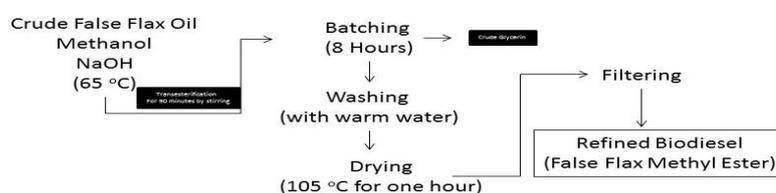
Figure 1: Biodiesel production flow diagram
