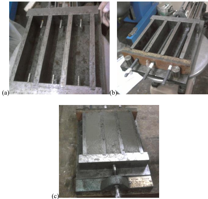
Fig. 3 Mold of specimens (a) Without reinforcement, (b) With reinforcement, (c) General appearance
