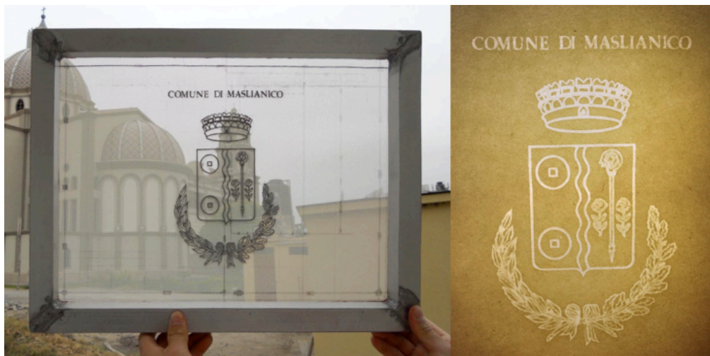
Visual 3. Left: The moulded mesh used to produce the paper with the watermark. Right: The watermark can be observed when paper is looked at in front of a light source. (Source: http://www.cartamanonelleande.org/IT/galleria_filigrane )
