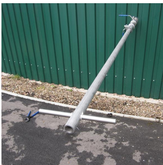
Fig 2. Measuring rod used for the velocity measurements
