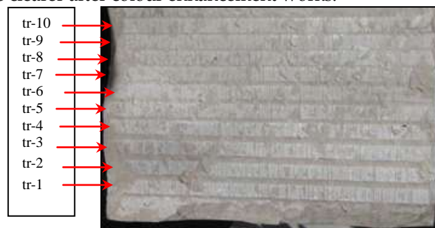
Figure 8. Drag bit traces on white marble surface; 12.7 mm wide drag bit started the cutting from left side of the specimen, (Cutting trace lengths were about 250 mm in average)
