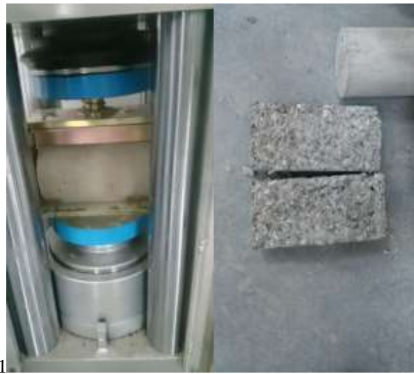
Figure 3. Split tensile test
