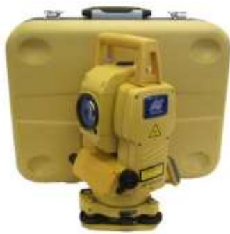
Figure 7.Topcon GPT – 3007 Reflektorless Total Station and Technical Specifications
