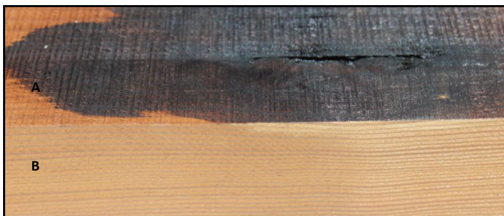
Figure 3 Release of resin on wood surface during thermal treatment. A. Wood surface with released resin from a resin pocket before sanding, B. The same wood surface after sanding
