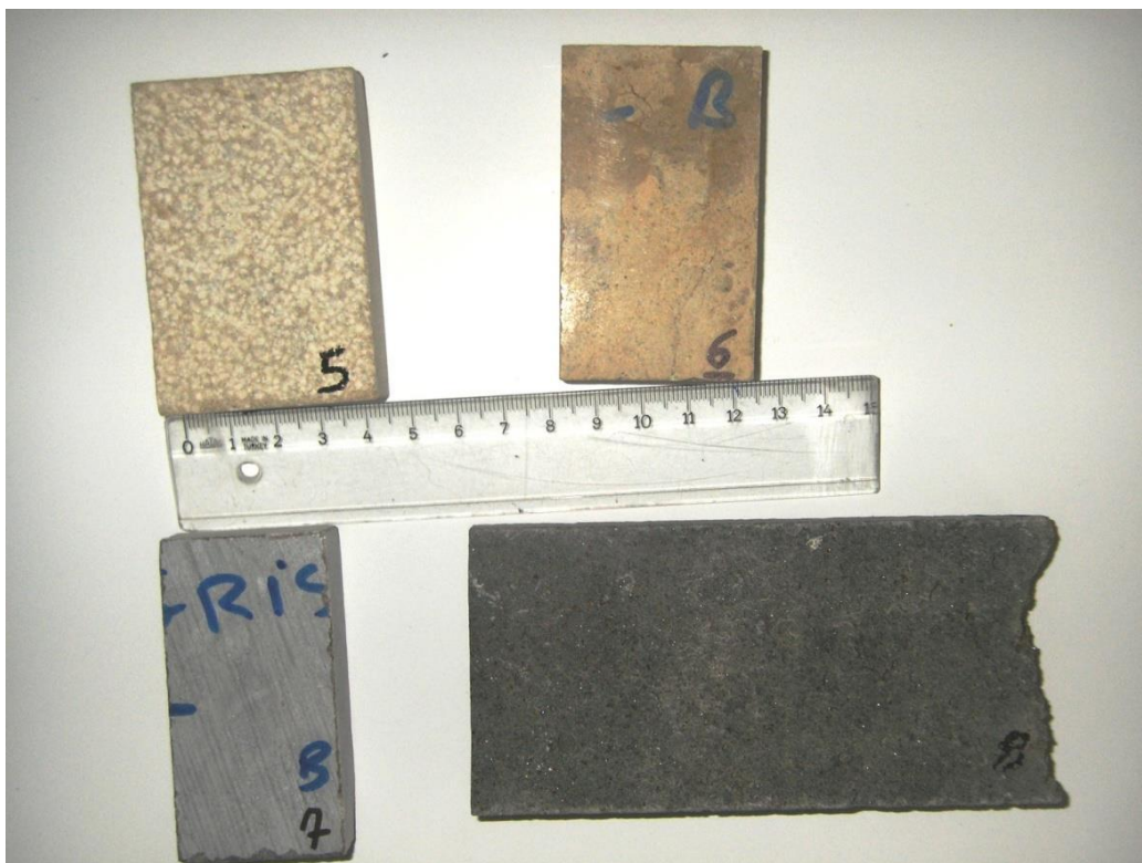
Figure 3. The studied samples of dolomitic limestones of Taza (5), Bejaad (6), and Gris (7), and Khenifra basalt (8).
