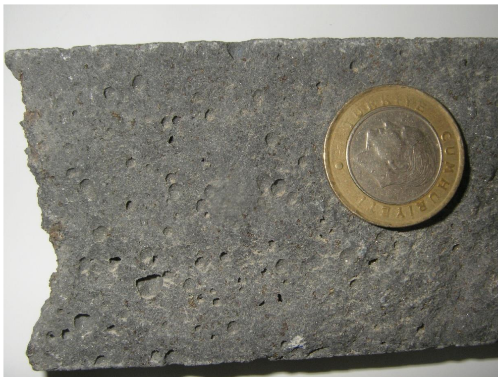
Figure 5. The studied sample of Khenifra basalt. The pores relatively more connected than all other samples (except Bir Jdid limestone).
