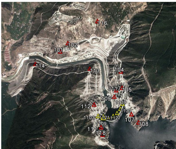
Figure 2. Distribution of reference and object points in Deriner dam
