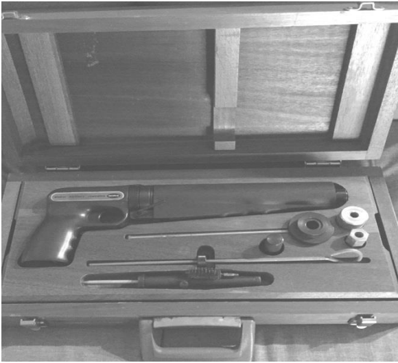
Figure 6. Windsor Probe Test equipments.
