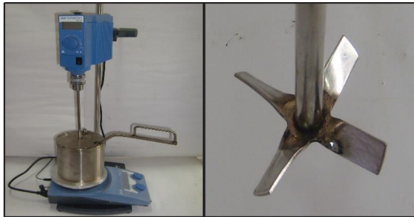
Fig 1. Modified bitumen mixer and mixing apparatus
