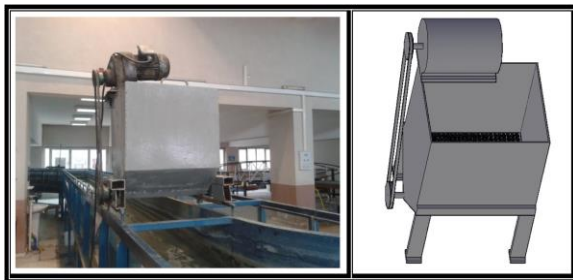
Figure 10. Portative machine that provide solid material supply to the channel.
