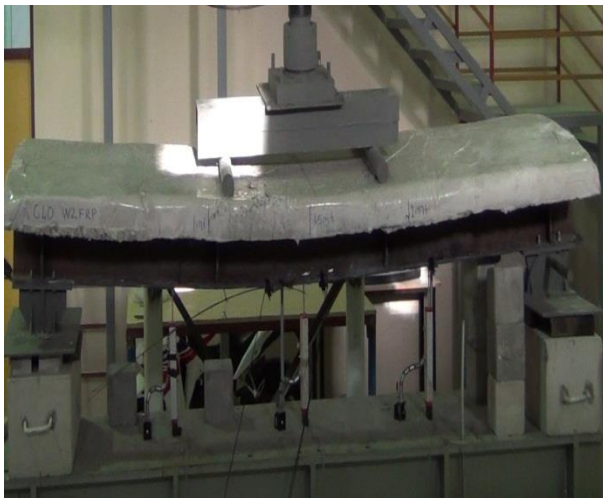
Figure 17. Deformed shape of the strengthened sample
