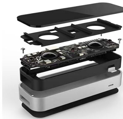
Fig. 2: Layer structure of the Leap Motion™
