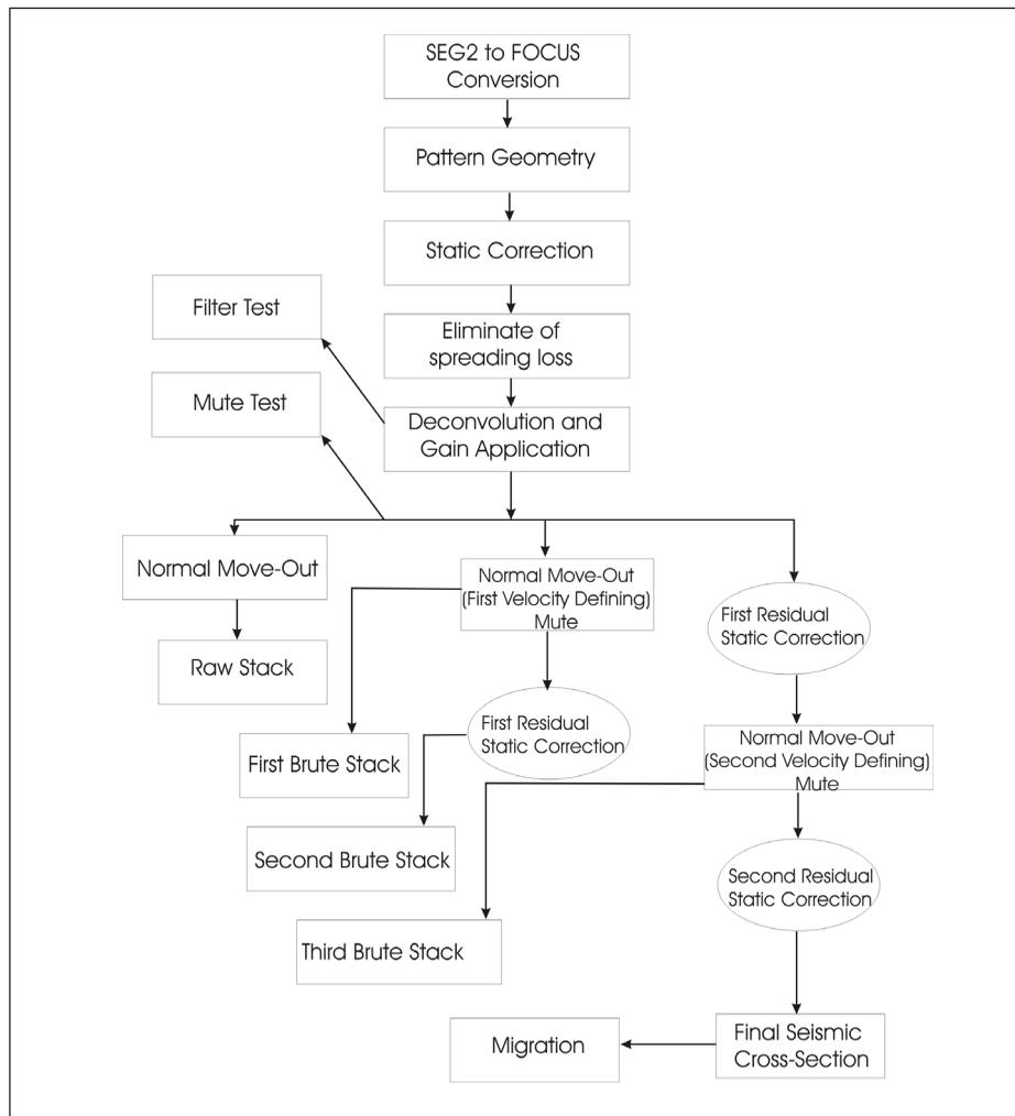
Figure 3- The process flow-chart of Afşin-Elbistan seismic data.
