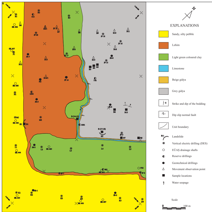
Figure 2- Geological and engineering geological map of the west face of the Kışlaköy open pit (Akbulut et al 2007).
