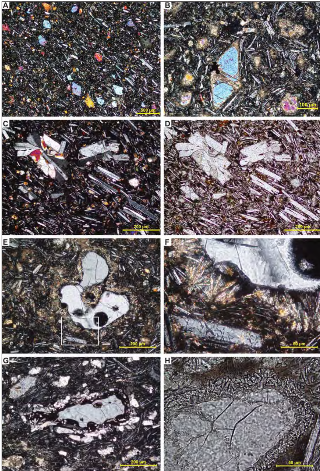
Figure 14- Microphotos reflecting mineralogical and petrographical characteristics of Karaburun volcanites. A) Hypocrystalline porphyric texture in which olivine phenocrysts and oriented plagioclase microliths are observed; B) Calcification in euhedral olivine phenocryst; C, D) orientation and glomeroporphyritic texture in plagioclase microliths and microphenocrysts (C: cross nicol; D: planonicol); E, F, G, H) Quartz crystals which subjected to magmatic corrosion were occasionally surrounded by radiate acicular or anhedral pyroxene microliths.
