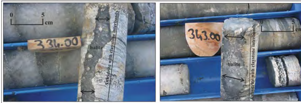
Figure 15- Rocksalt which was deposited into sediment; a) Balıbağı-1 drill, b) Yenidoğan-1 drill.
