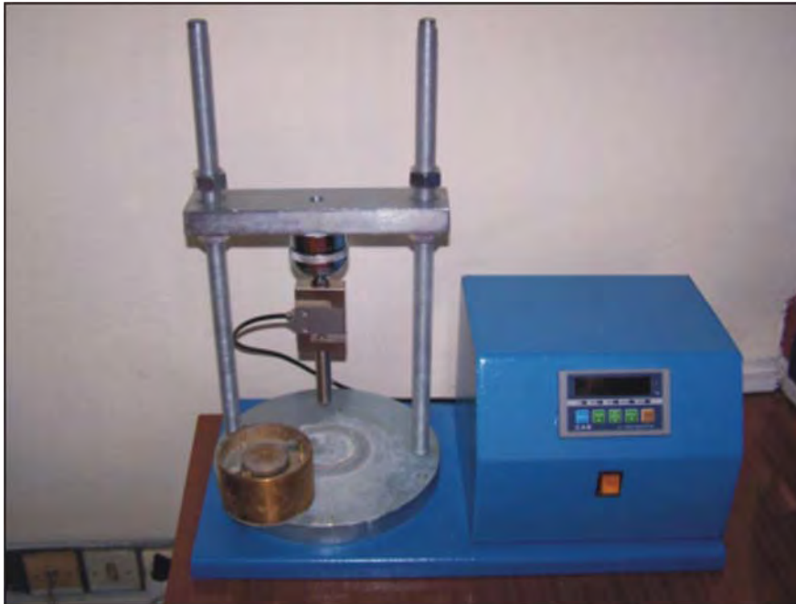
Figure 1- Constant volume swell test apparatus.
