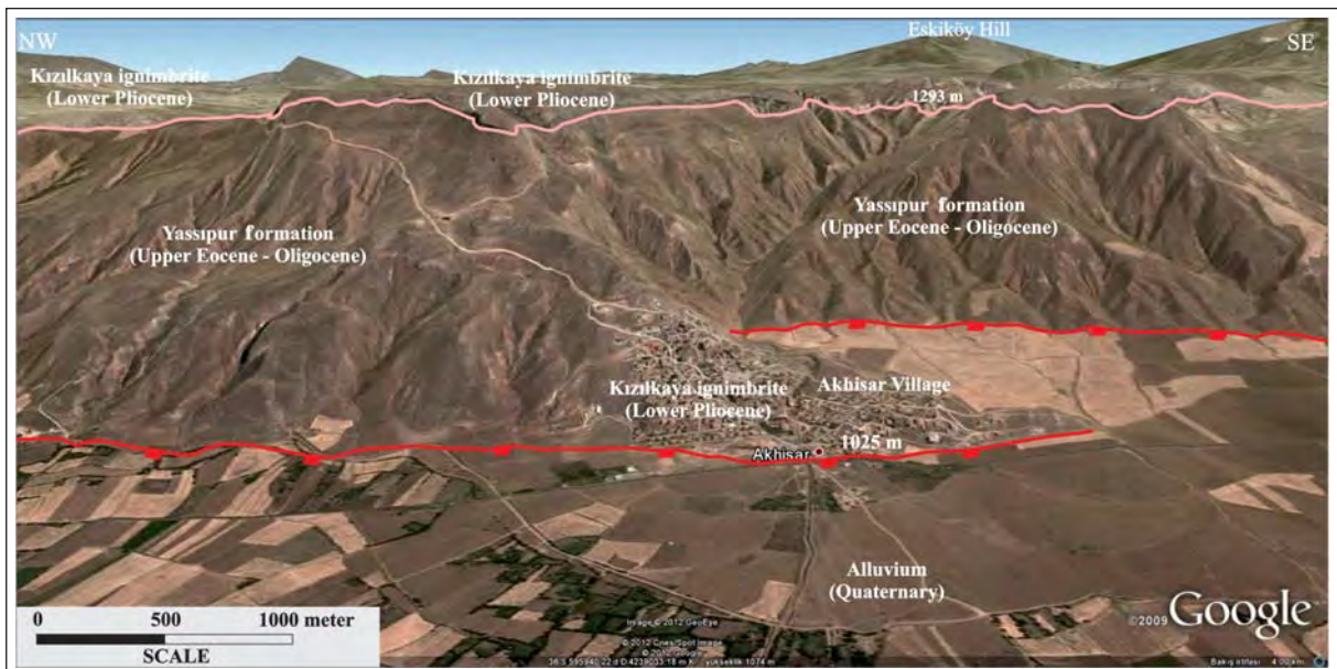
Figure 38- Processed Google Earth image showing stratigraphic relations of units around the Akhisar village (vertical scale three times exaggerated, view to NE with oblique angle)
