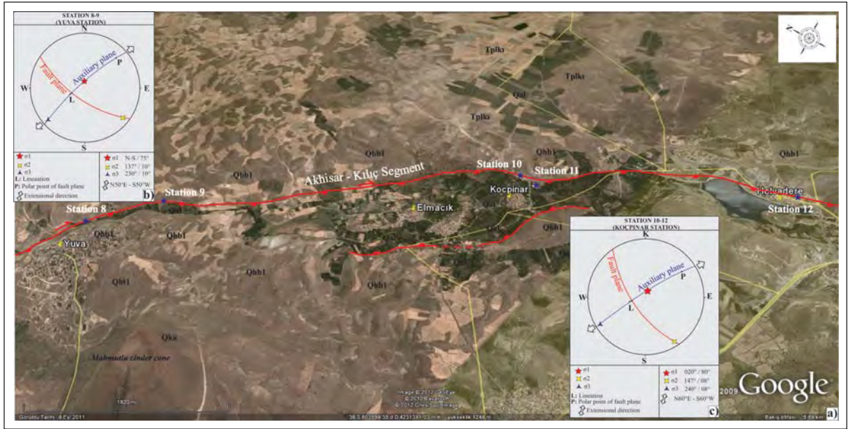
Figure 20- a) Google Earth view of central part of the Akhisar-Kılıç segment (see Figure 18 for location) (vertical scale three times exaggerated, view to NE). Tmü: Ürgüp fm, Tplk1: Kızılkaya Ignimbrite, Qka: Karataş Volcanites, Qht1: First-stage air fall and flow tuffs of the Hasandağ Volcanites, Qal: Alluvium, Stations 8, 9, 10, 11 and 12: structural observation site on the Akhisar-Kılıç segment, b) Presentation on the lower hemisphere of Schmidt net projection of single-plane solution of fault plane no 4 measured at Station 4 (Yuva station) in accordance with Marshak and Mitra (1988). The arrow on the fault plane shows the relative movement direction of hanging wall; c) Presentation on the lower hemisphere of Schmidt net projection of single-plane solution of fault plane no 4 measured at Stations 10-11 (Koçpınar station) in accordance with Marshak and Mitra (1988). The arrow on the fault plane shows the relative movement direction of hanging wall.
