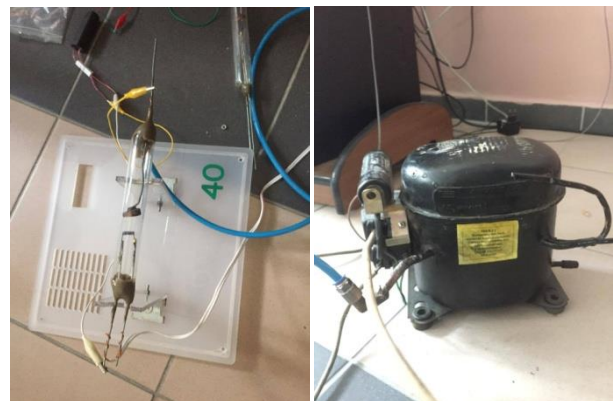
Figure 8. Vacuum application to the X-ray tube
