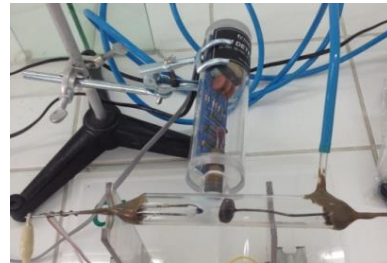
Figure 12. Geiger-Muller counter and X-ray tube
