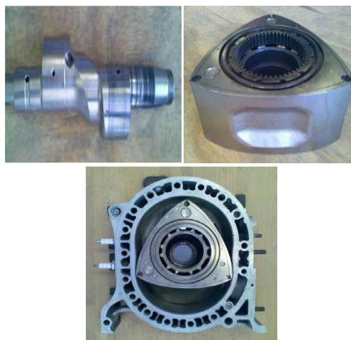
Figure 4. Wankel Rotary Engine Eccentric Shaft, Bathtub Face of Wankel Rotor, Wankel Rotor and Stator [7]
