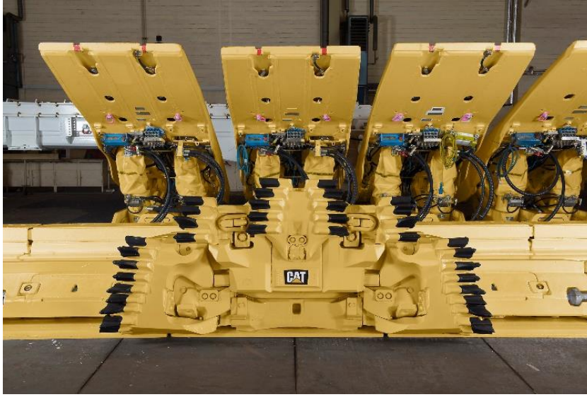
Şekil 3. Tam mekanize kazı sistemi (Cat.com., 2017) Figure 3. Fully Mechanized Excavation System
