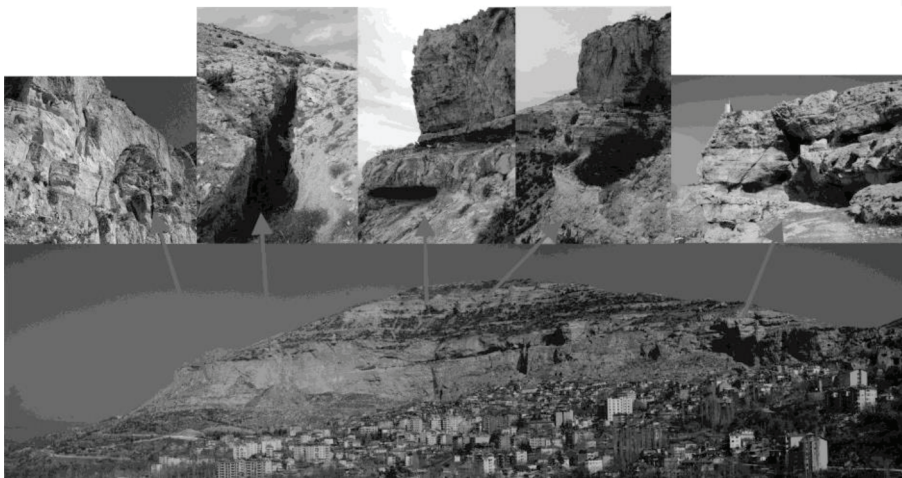
Figure 11. Photographs showing hanging blocks and their location in the study area (not to scaled).
