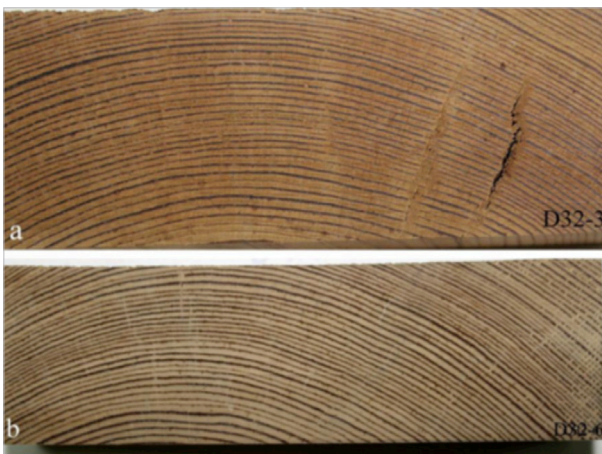
Figure 6. a, b. Thermo-D applied heartwood samples (a) internal crack formation, (b) cupping
