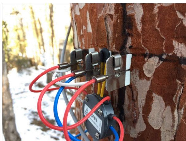
Figure 2. Electrodes, needle type thermocouples, isolator band and electric supplier hooks on the tree trunk
