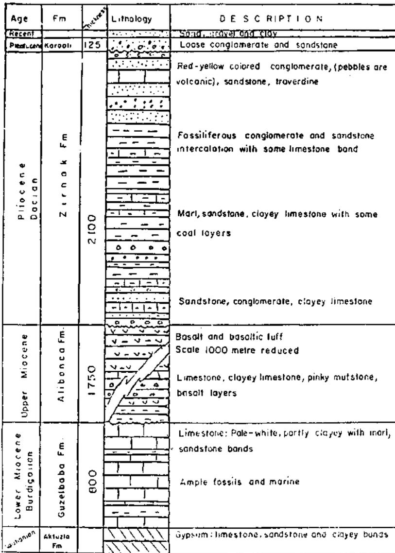
Fig. 8 - Generalized stratigraphic section of the Zirnak area (collected from Birgili, 1968; Şenalp, 1966 and İlker, 1966a).
