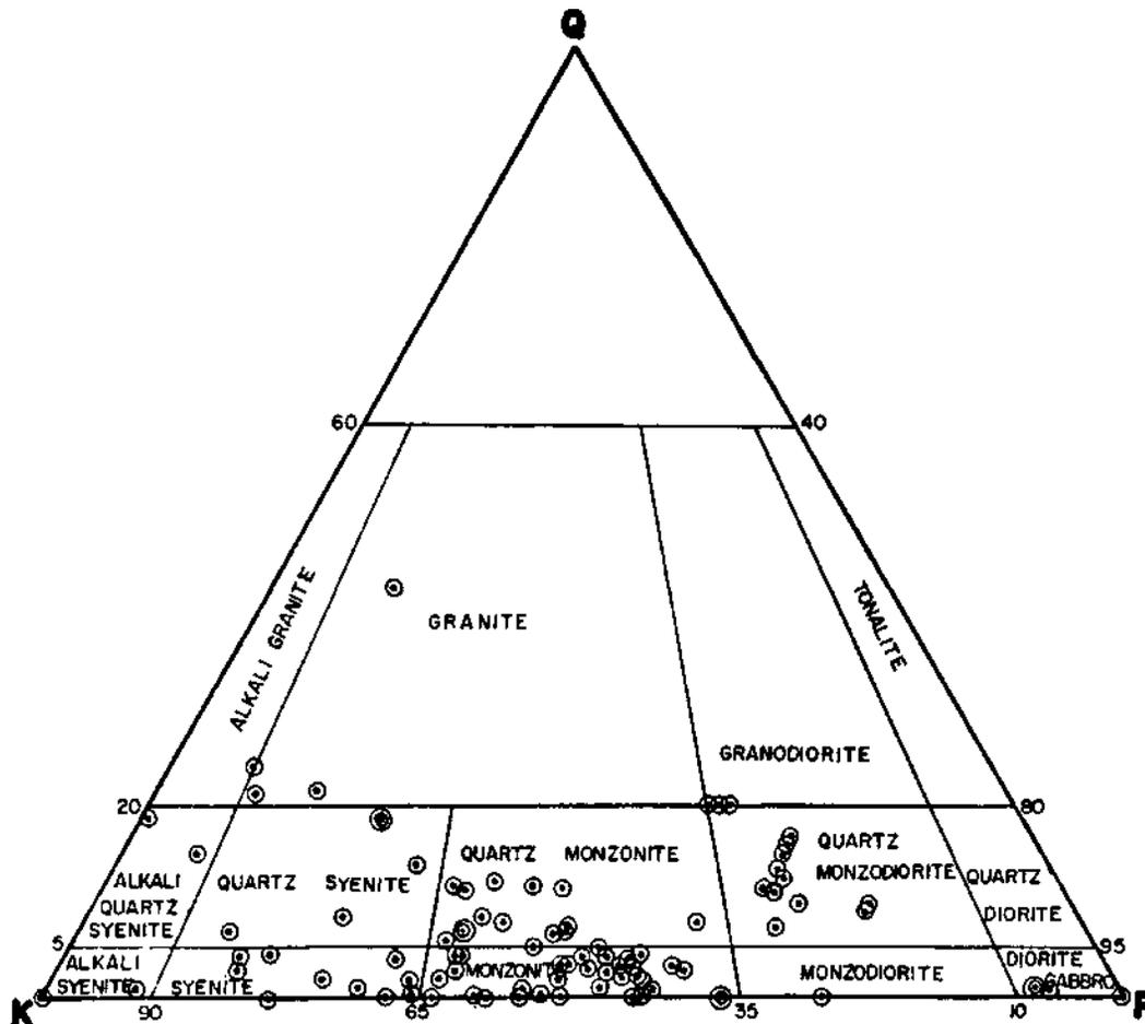
Fig. 12 - Distribution of Divriği granitic rocks in Streckeisen diagram (1976).
