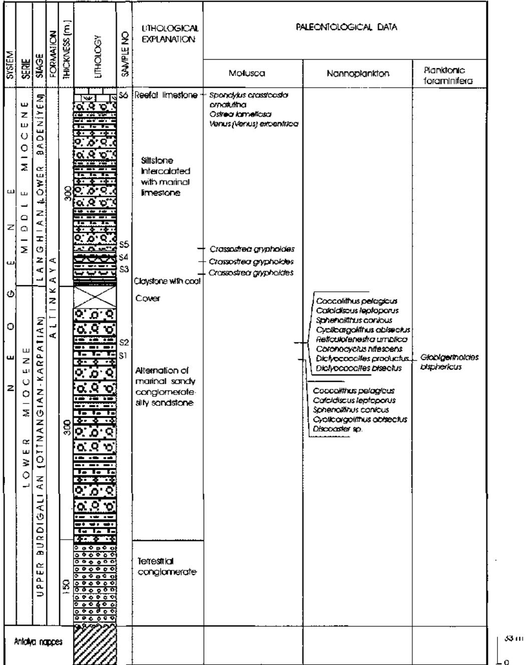
Fig. 6- The Altinkaya stratigraphic section measured in the Altinkaya formation (EE')
