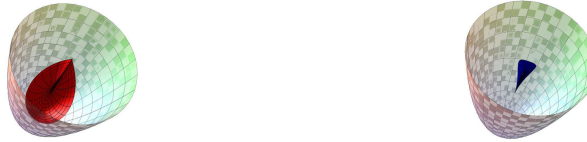
Figure 1.3: Two reflected caustics of elliptic paraboloid in case of incident rays parallel non-parallel to the axis of symmetry
