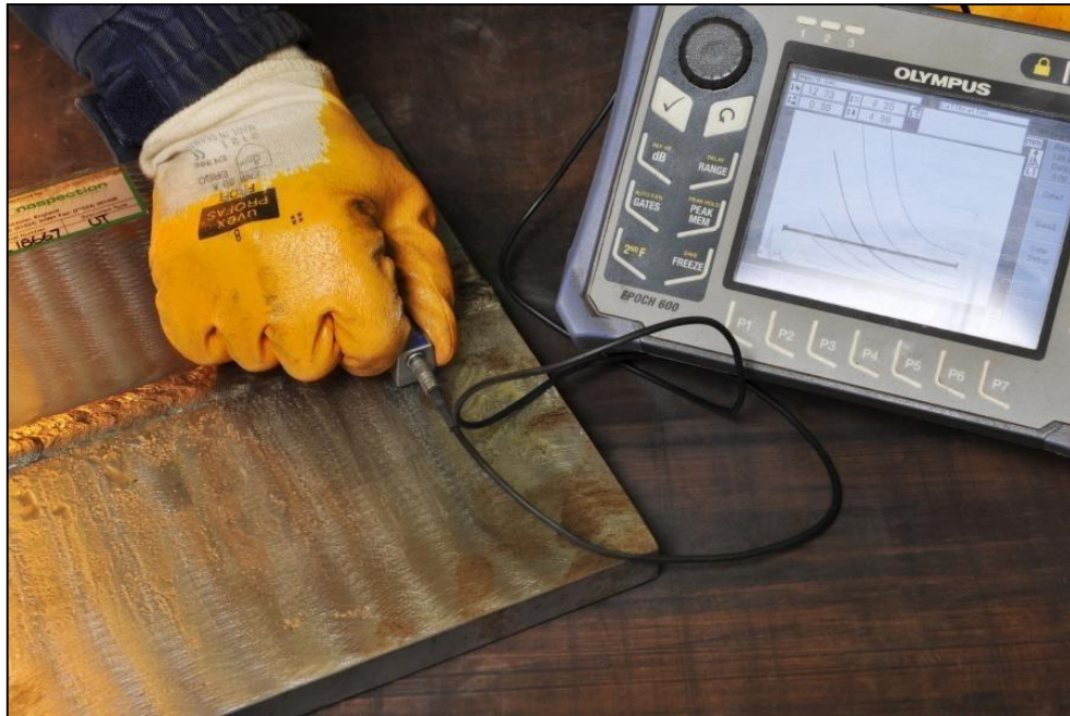
Fig. 1. The Ultrasonic Equipment
