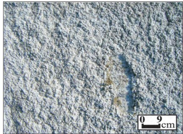
Figure10 - Weak, efflorescence mineralization surface representing gypsum + calcite+bloedite zone.
