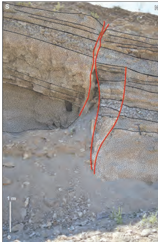
Figure 18- Section-KAR 1 is a 4 m-thick sequence consisting of a flat-lying upper unit of interbedded sandstone and conglomerate. See figure 1 for location.
