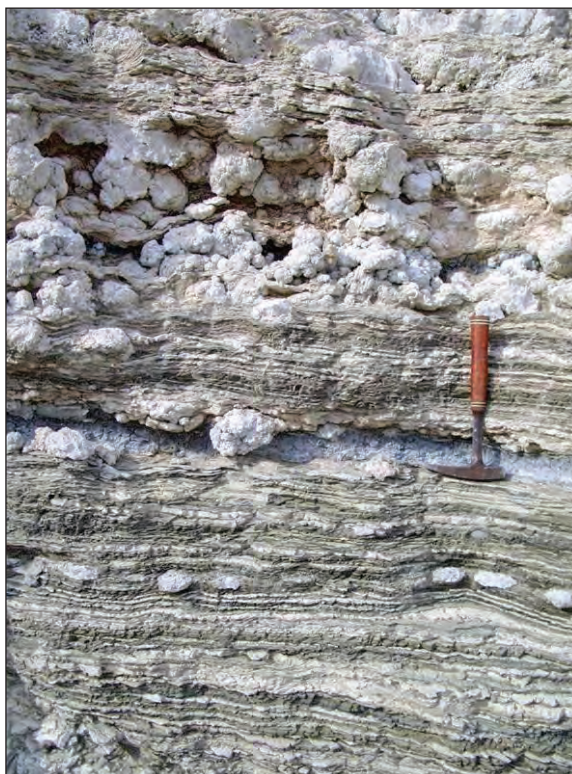
Figure 15- Colemanite nodules in varying sizes intercalated with associated sediments, Tülü open pit mine deposit, Bigadiç, Turkey.
