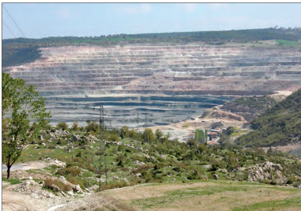
Figure 22- Section of borate zone interbedded with clay and tuff, and limestone overburden, Espey deposit, Emet, Turkey.
