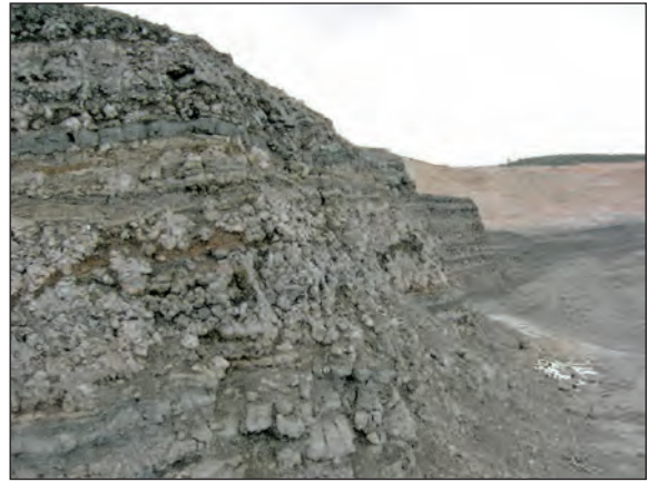
Figure 14- Sediments in the borate lakes showing clear evidence of cyclicity, and volcanic tuff intercalations with the sediments in the borate unit. Colemanite nodules occurring within clayey-tuffaceous matrix, Hisarcık open pit mine, Emet, Turkey.
