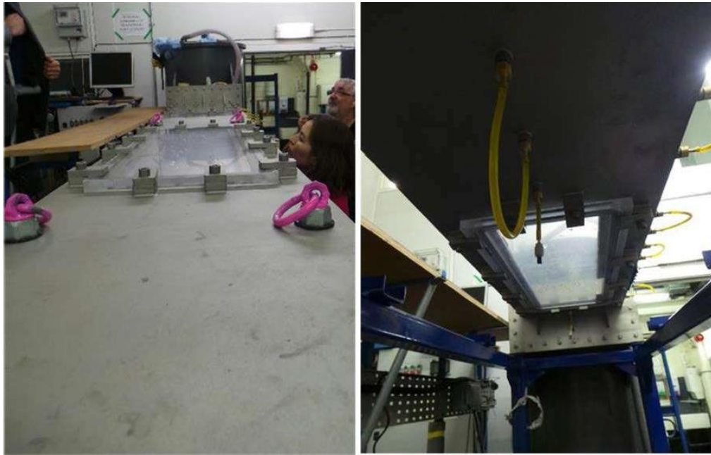
Fig. 8. Two parallel smooth test panels (Surface A and its replicate) in place, top panel (left); bottom panel (right)
