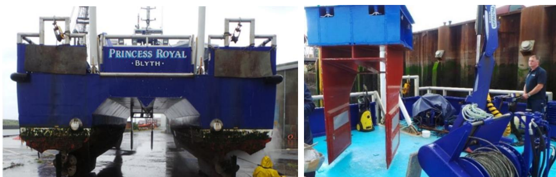
Fig. 7. UNEW RV- The Princess Royal (left) and its strut arrangement to carry fouling plates (right)
