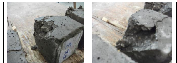
Figure 5. Image of Concrete Specimen containing 10% Nut Shell Ash Additive
