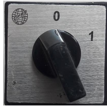
Figure 9. Manual and automatic option for height level arrangement
