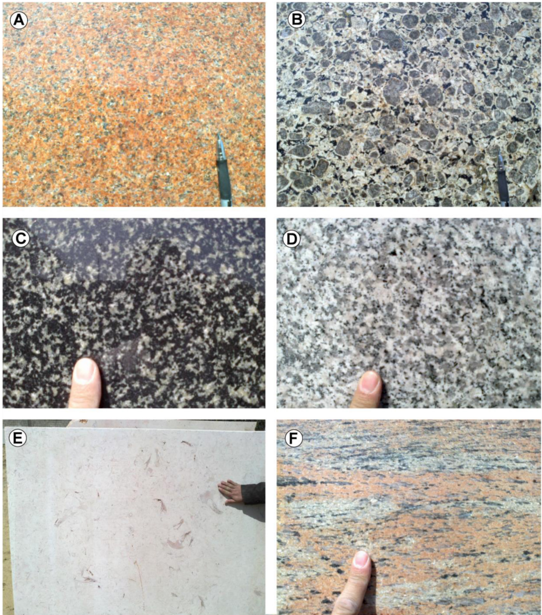
Figure 3. Some samples of rocks used in construction purposes in Gaza Strip. A, B, C and D represent plutonic igneous rocks. E and F represent metamorphic rocks.
