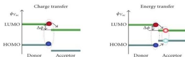
Figure 5. Load and energy transfer in organic solar cell
