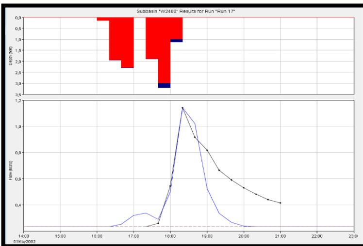
Figure 9. Observed and simulated hydrographs in 2002.
