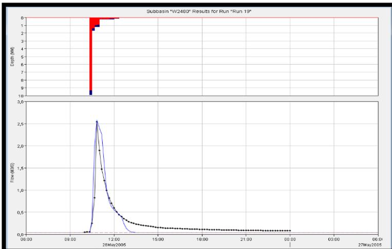
Figure 10. Observed and simulated hydrographs in 2005.
