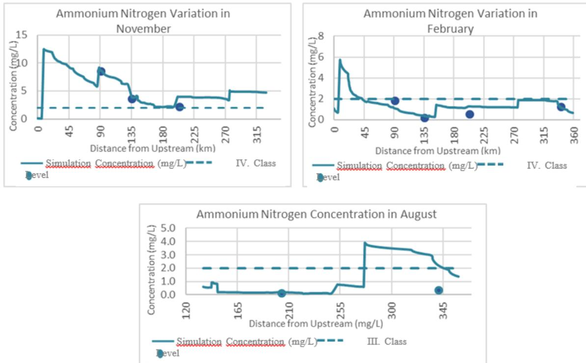
Figure 7. November, February and August NH<sub>4</sub>N Concentration through the main river branch.
