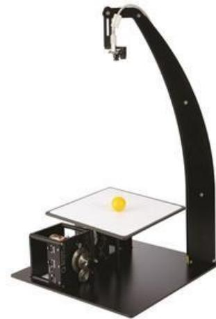
Fig.2. Ball and plate system made by QUANSER [27].
