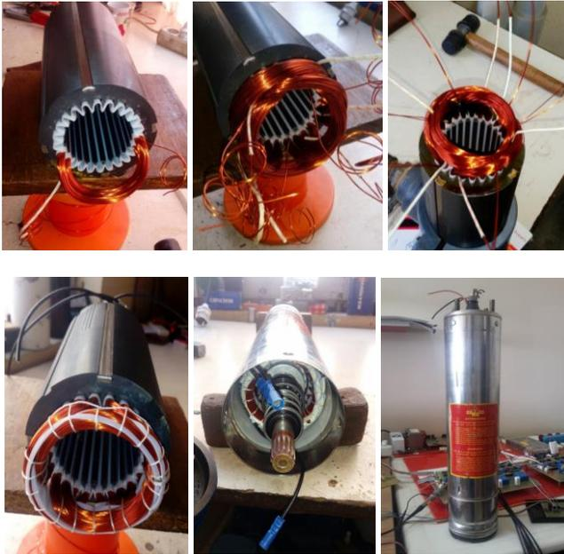
Figure 6. The photos related to motor winding process
